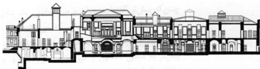
Fig. 3. Longitudinal section of the former National Assembly building showing its structural condition and vulnerability.
