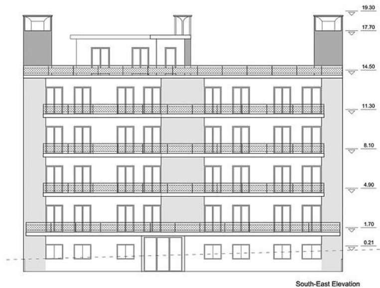
Fig. 8. South elevation of the case study building showing the three wind-catchers integrated at the building core on top of the light wells [12].
