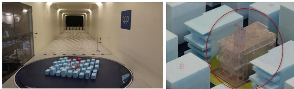
Fig.15. Simulation of a building with windcatchers (Inside the red circle) located in an urban environment.
